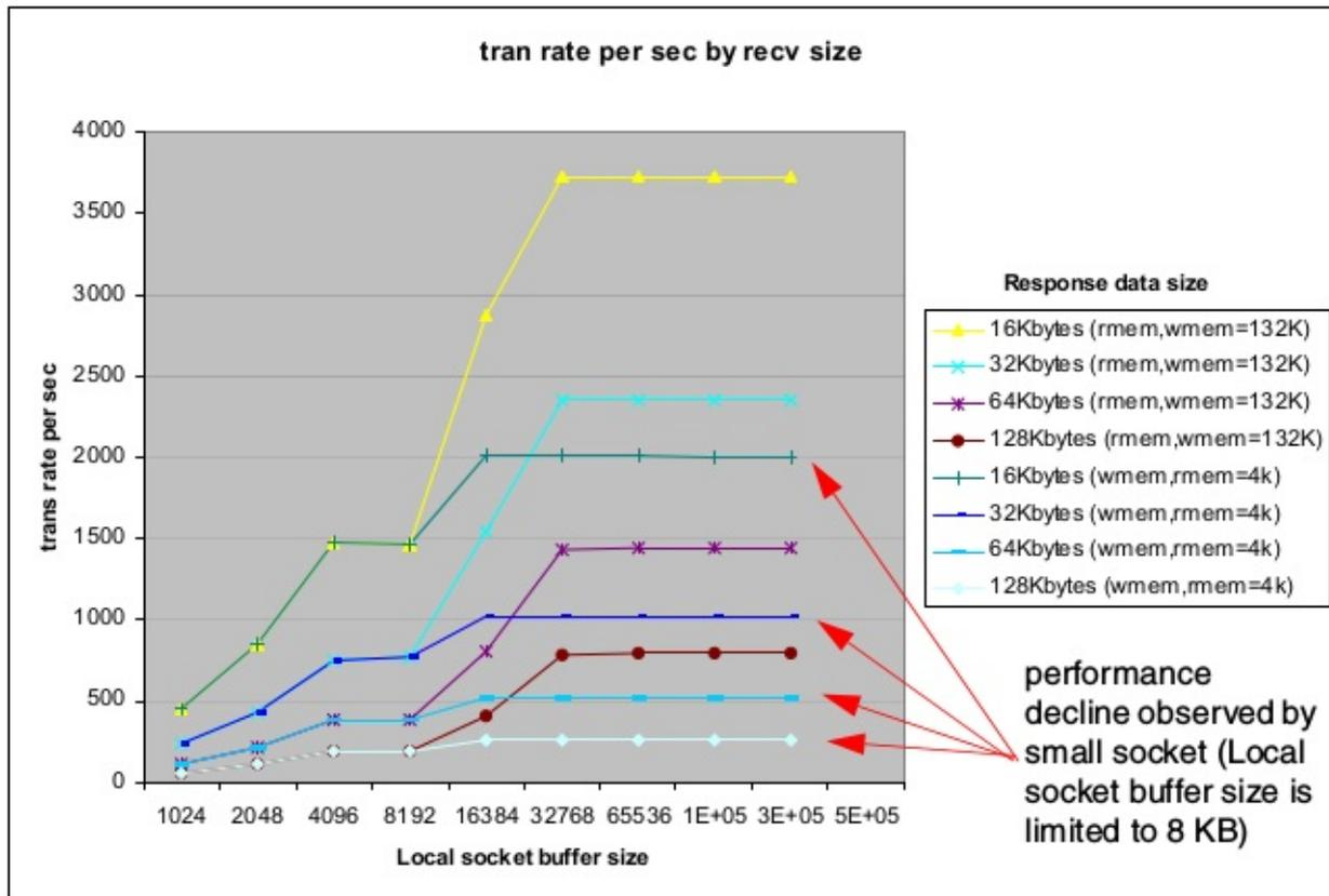
Figure 4-16 Comparison with socket buffer 4 KB and 132 bytes
