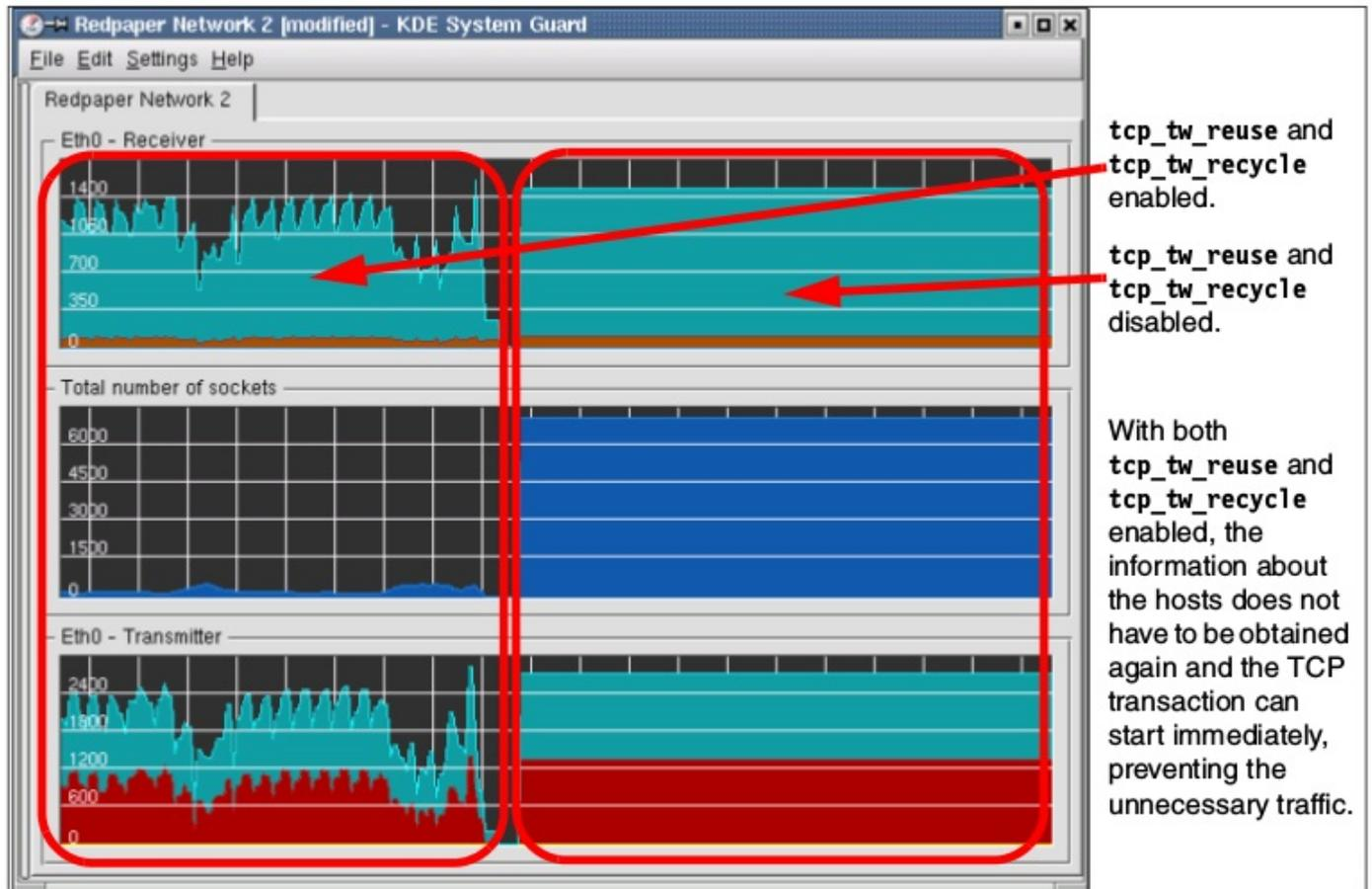
Figure 4-17 Parameters reuse and recycle enabled (left) and disabled (right)
