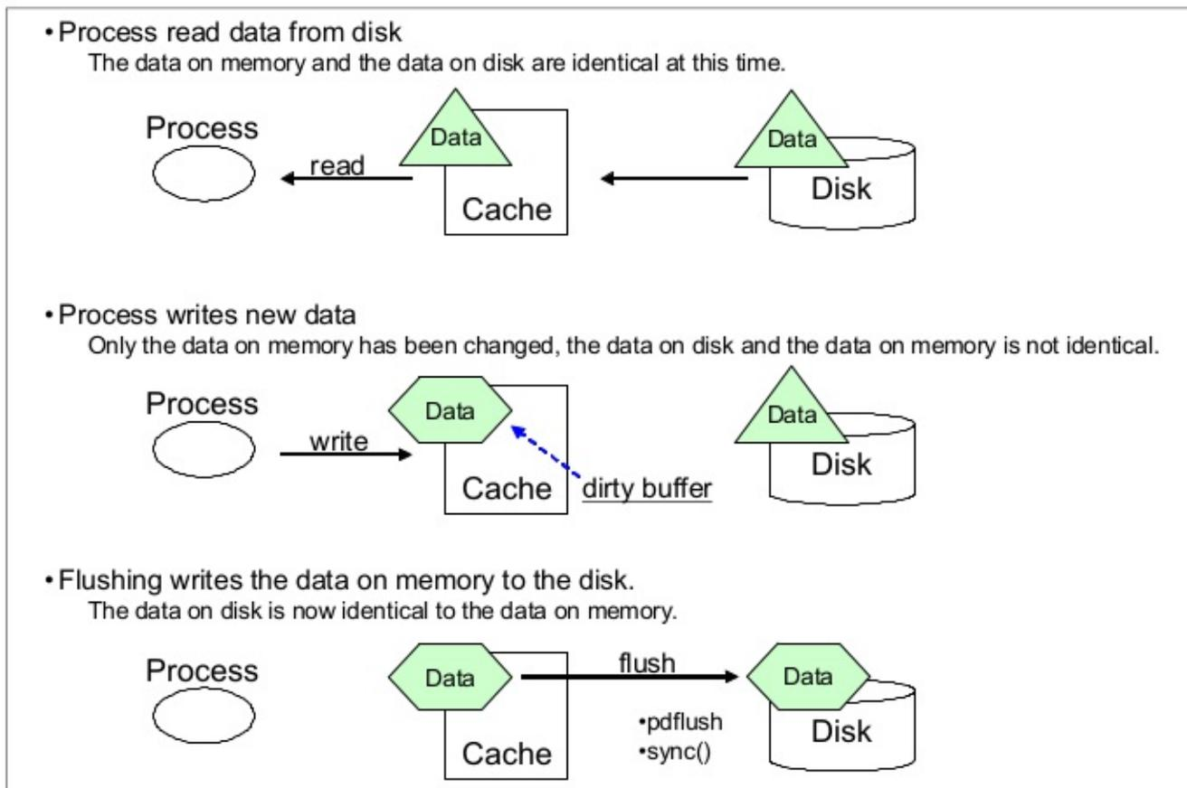
Figure 1-21 Flushing dirty buffers
