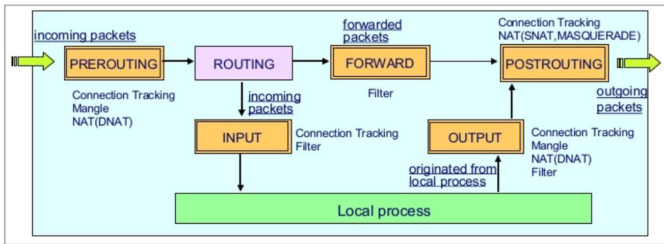
Figure 1-26 Netfilter packet flow
