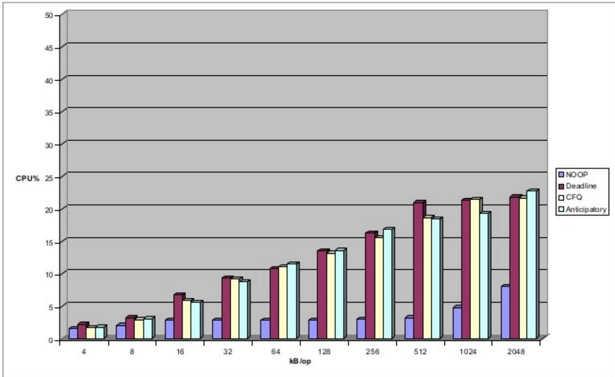
Figure 4-8 CPU utilization by I/O elevator (asynchronous)
