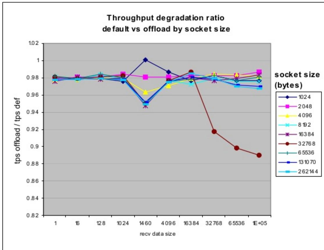
Figure 4-21 Throughput degradation by offloading
