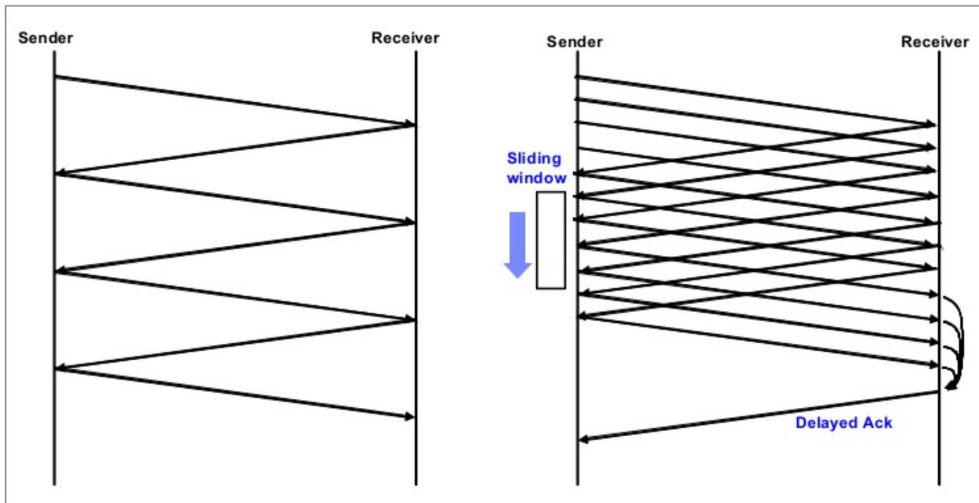
Figure 1-29 Sliding window and delayed ack
