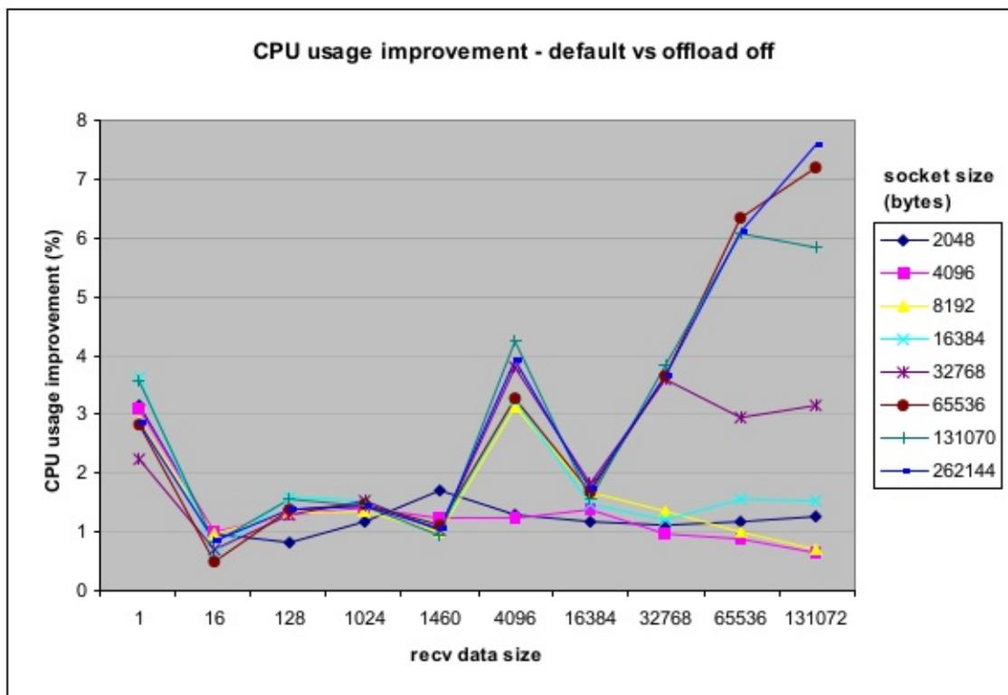
Figure 4-20 CPU usage improvement by offloading
