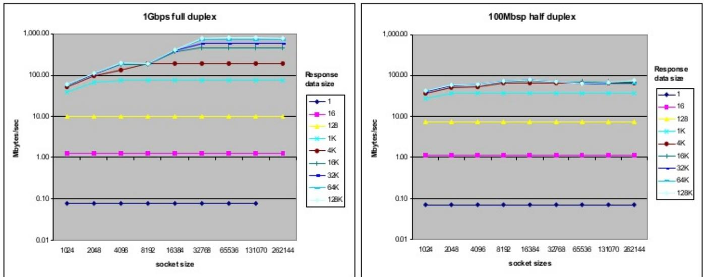
Figure 4-15 Performance degradation caused by auto negotiation failure
