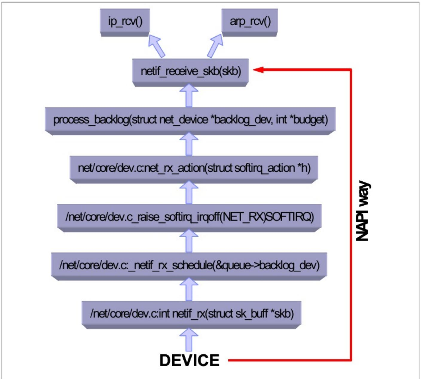
Figure 1-25 The Linux network stack
