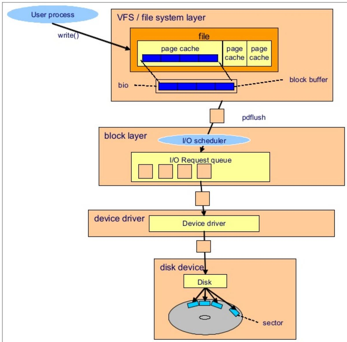
Figure 1-18 I/O subsystem architecture
