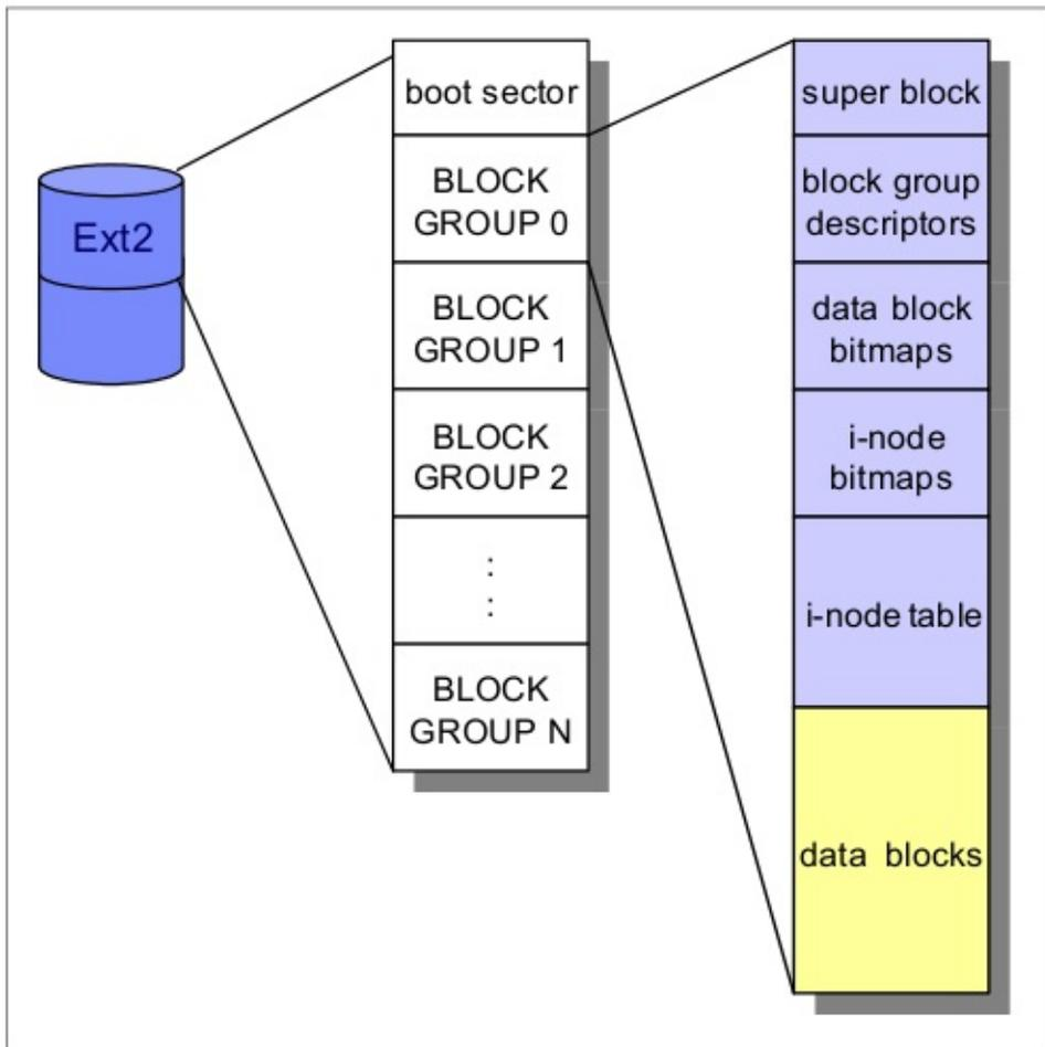
Figure 1-16 Ext2 file system data structure
