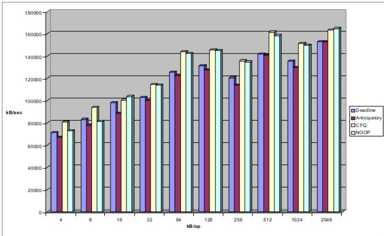
Figure 4-7 Random read performance per I/O elevator (synchronous)
