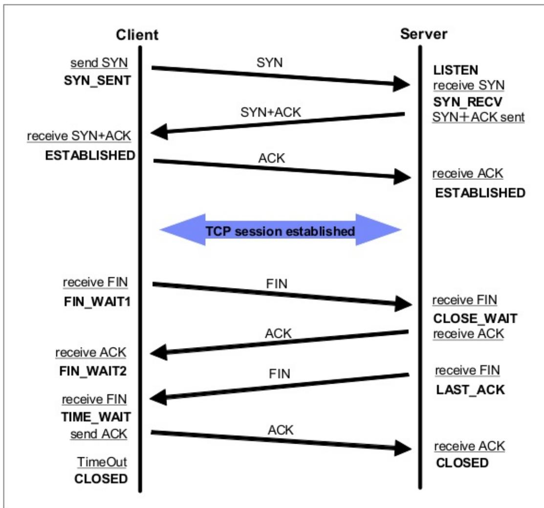
Figure 1-27 TCP 3-way handshake
